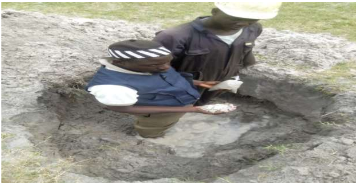
Plate 1b: photograph of trial pit showing the collection disturbed samples of 0.5m- 2.5m Ilaje Water Samples collected from the two communities of Ilaje and Irele
